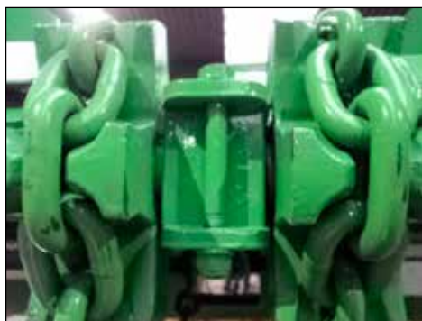
Moulded gearwheels and chains
